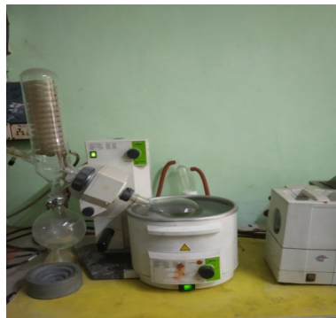
Fig 4: Condensation of extracts in Rotary vacuum Evaporator
